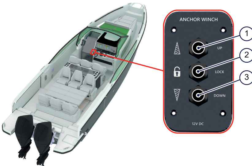
Figure 4.10 - Anchor winch control panel
