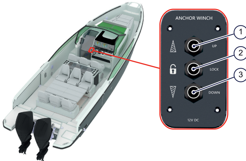
Figure 4.10 - Anchor winch control panel
