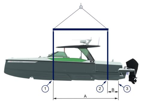
Figure 4.25 - Lifting points
