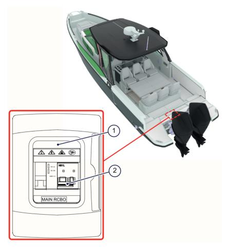
Figure 4.16 - Air-conditioning fuse panel
