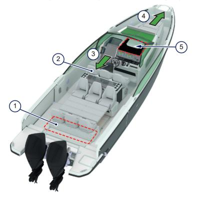
Figure 4.21 - Safety equipment and emergency exits
