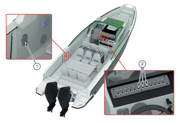
Figure 5.7 - Manual bilge pump and automatic bilge pump controls
