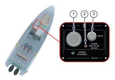
Figure 4.12 - High bilge alarm control panel
