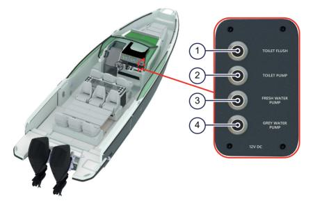
Figure 4.11 - Toilet compartment control panel
