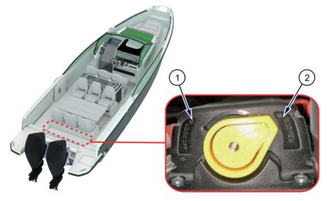
Figure 5.3 - Battery pack safety relay switch ON / OFF
