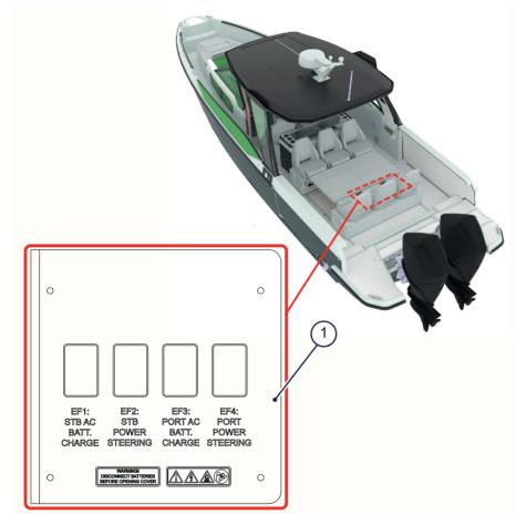
Figure 4.15 - Heavy-duty fuse panel
