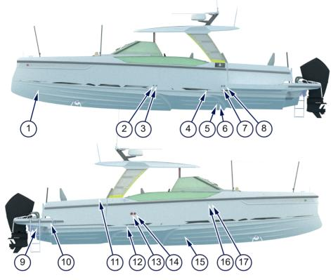
Figure 4.26 - Hull openings
