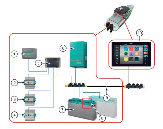
Figure 5.2 - Generator replacement system as a part of the power package system
