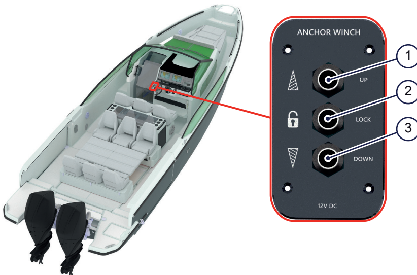
Figure 4.5 - Anchor winch control panel
