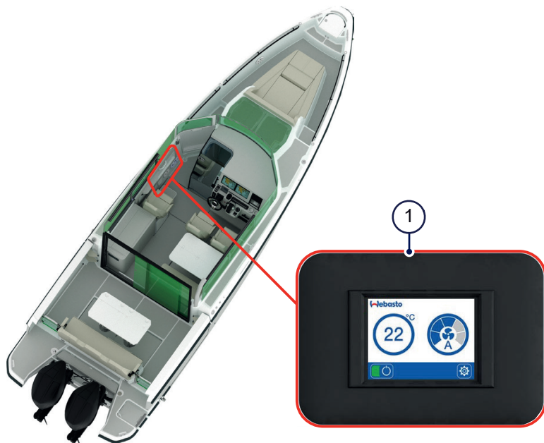
Figure 4.20 - Temperature control panel
