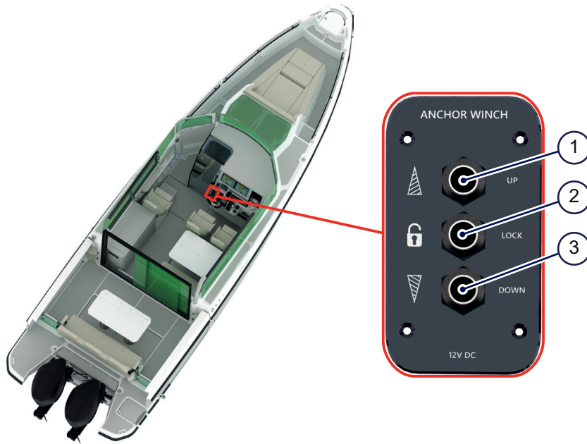
Figure 4.10 - Anchor winch control panel
