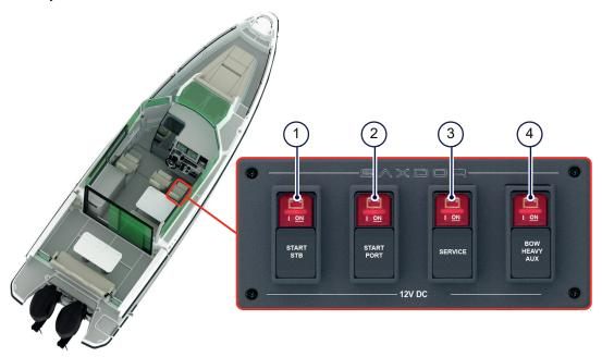
Figure 4.19 - Battery control panel
