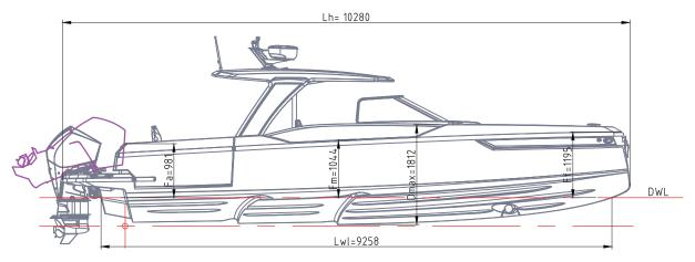
Figure 8.1 - Saxdor 320 GTC dimensions, side view
