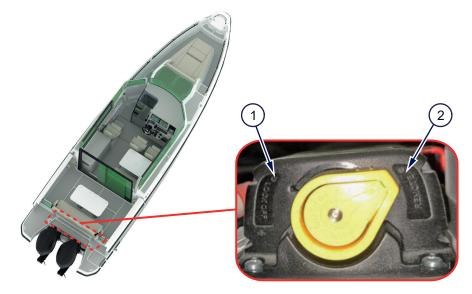
Figure 5.3 - Battery pack safety relay switch ON / OFF
