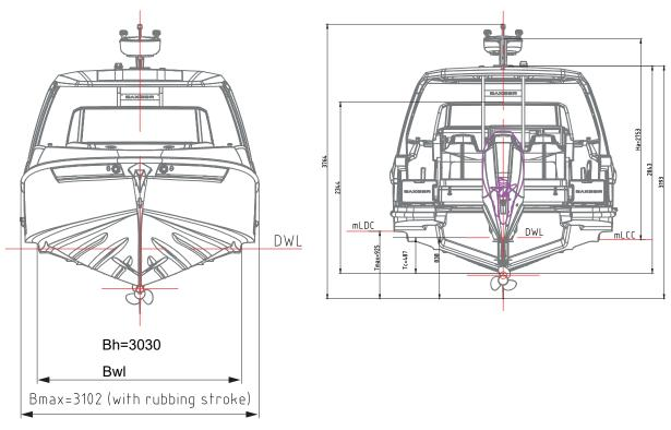
Figure 8.3 - Saxdor 320 GTC dimensions, bow and aft view
