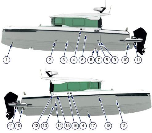
Figure 4.29 - Hull openings
