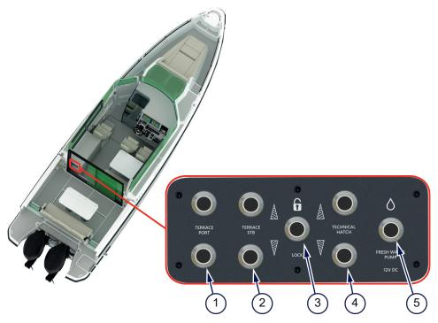
Figure 4.14 - Side terrace control panel
