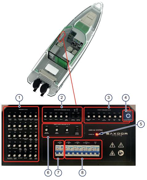
Figure 4.16 - Front cabin fuse panel
