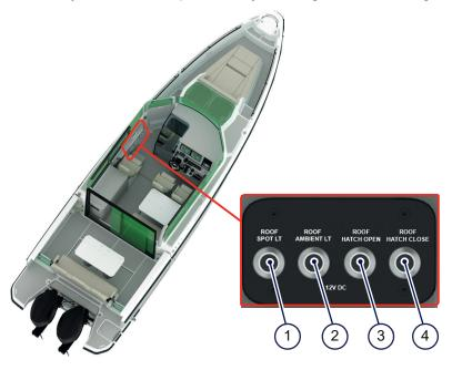
Figure 4.15 - Roof control panel
