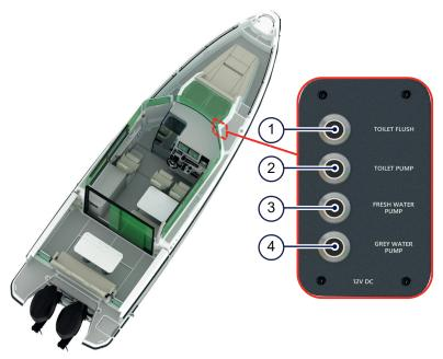
Figure 4.12 - Toilet compartment control panel
