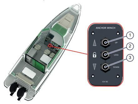
Figure 4.10 - Anchor winch control panel
