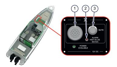
Figure 4.13 - High bilge alarm control panel
