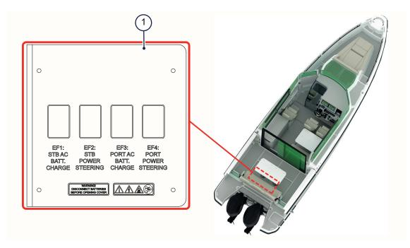
Figure 4.17 - Heavy-duty fuse panel
