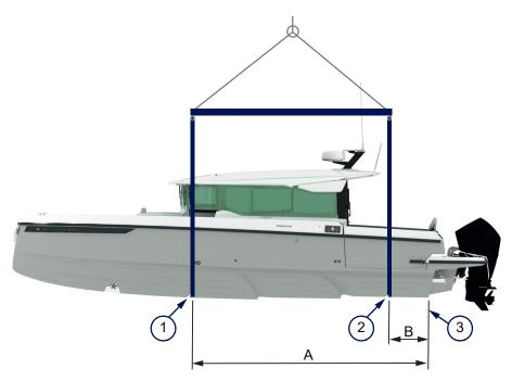
Figure 4.28 - Lifting points
