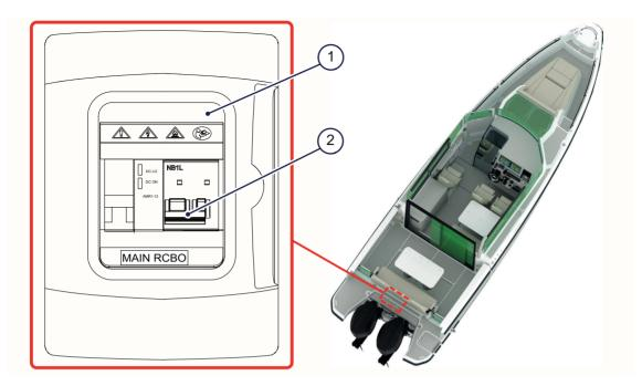
Figure 4.18 - Air-conditioning fuse panel
