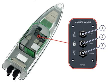
Figure 4.10 - Anchor winch control panel
