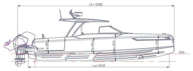
Figure 8.1 - Saxdor 320 GTC dimensions, side view
