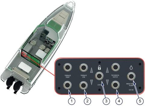
Figure 4.14 - Side terrace control panel
