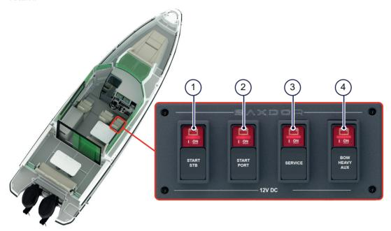
Figure 4.19 - Battery control panel
