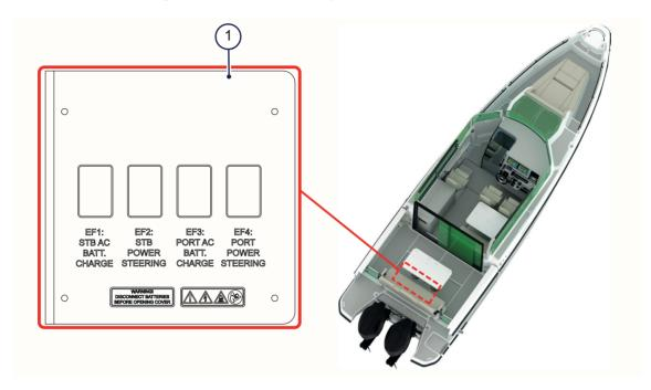
Figure 4.17 - Heavy-duty fuse panel
