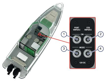
Figure 4.11 - Wiper control panel
