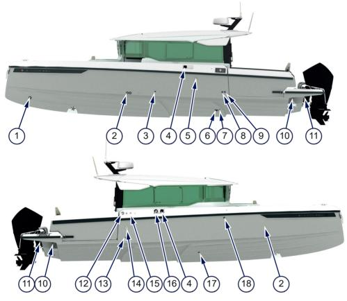
Figure 4.29 - Hull openings
