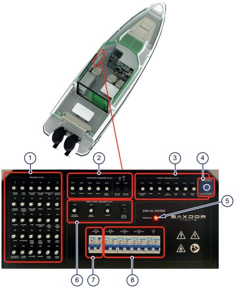
Figure 4.16 - Front cabin fuse panel
