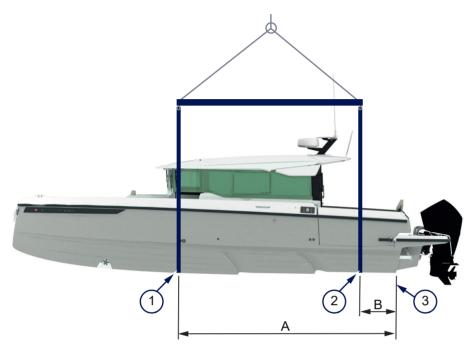
Figure 4.28 - Lifting points
