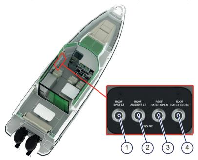
Figure 4.15 - Roof control panel
