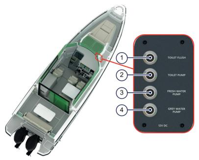
Figure 4.12 - Toilet compartment control panel
