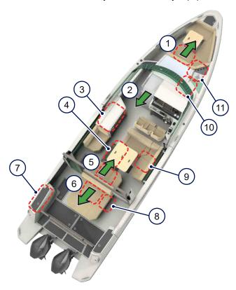
Figure 4.22 - Safety equipment and emergency exits
