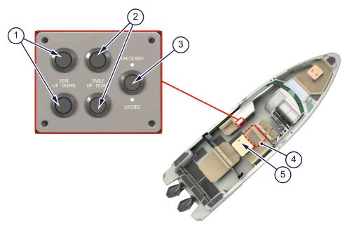
Figure 4.11 - Cockpit table control panel
