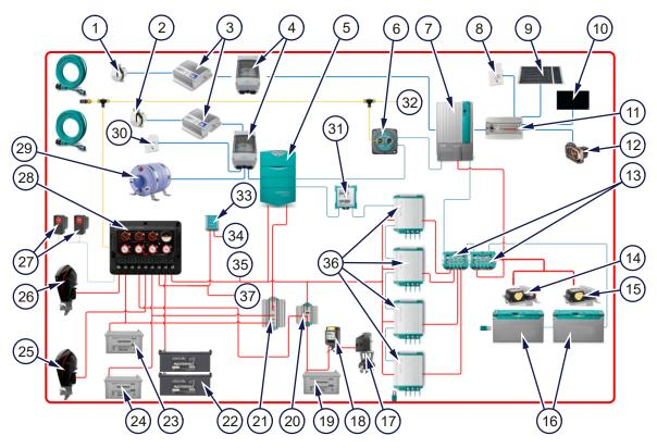
Figure 5.4 - Electrical system and generator replacement system
