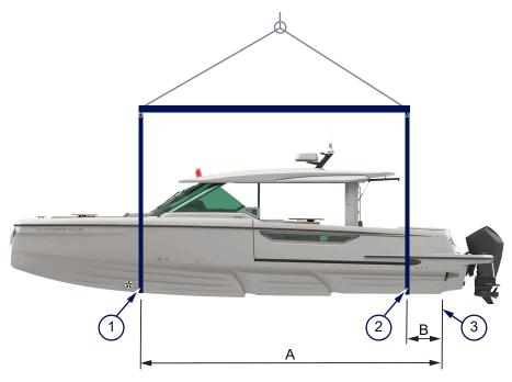
Figure 4.26 - Lifting points
