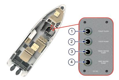
Figure 4.12 - Toilet compartment control panel
