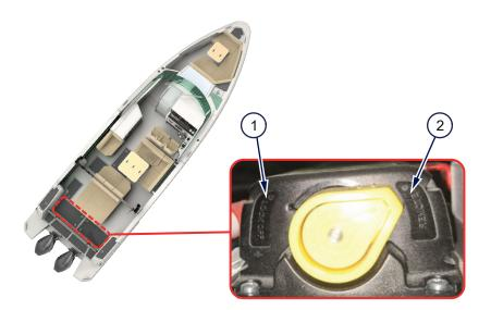
Figure 5.3 - Battery pack safety relay switch
