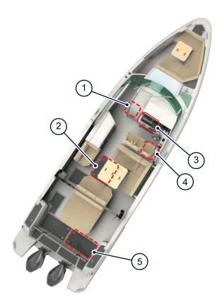
Figure 5.7 - Manual and automatic bilge pumps and controls
