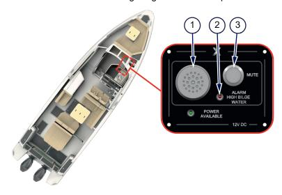
Figure 4.13 - High bilge alarm control panel
