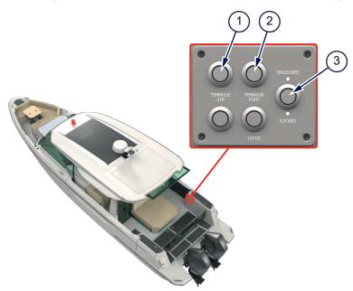
Figure 4.14 - Side terrace control panel
