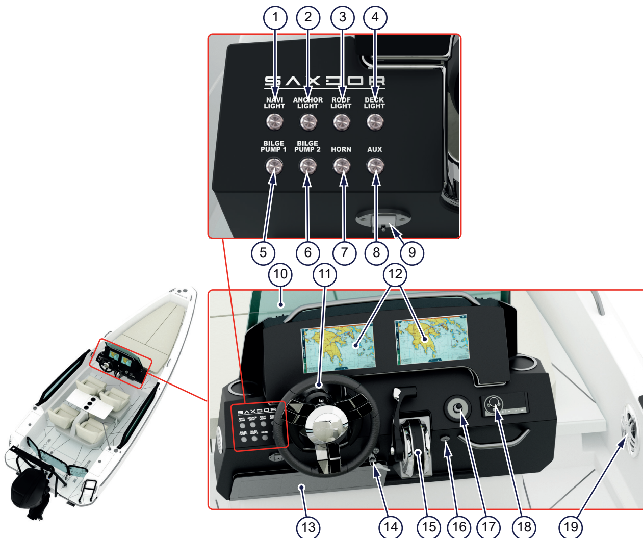
Figure 4.7 - Helm station controls
