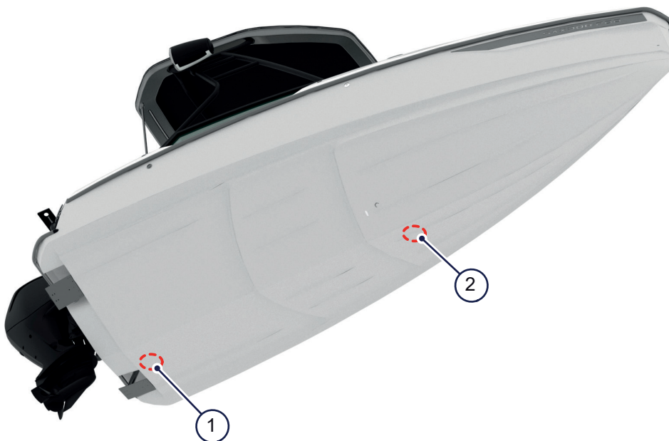
Figure 5.4 - Automatic bilge pumps
