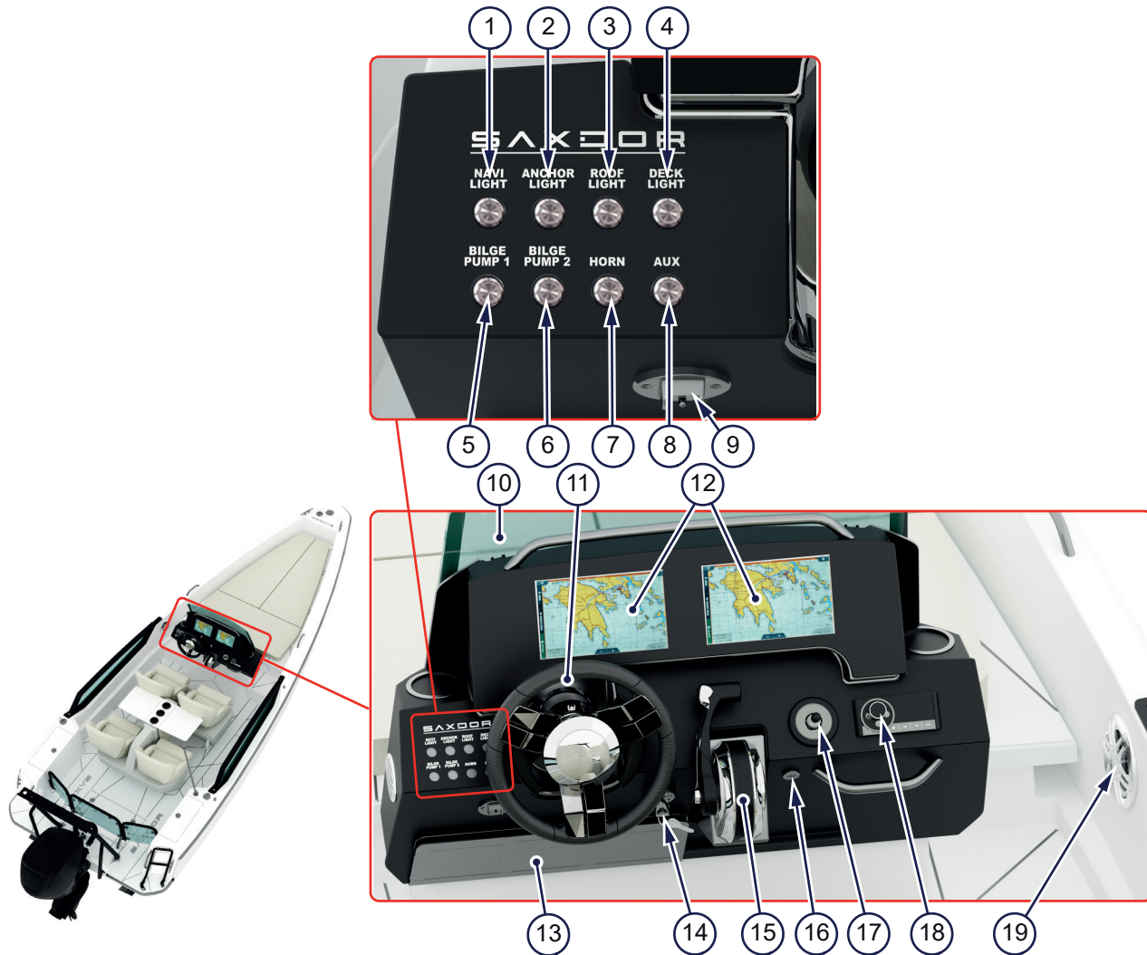
Figure 4.7 - Helm station controls
